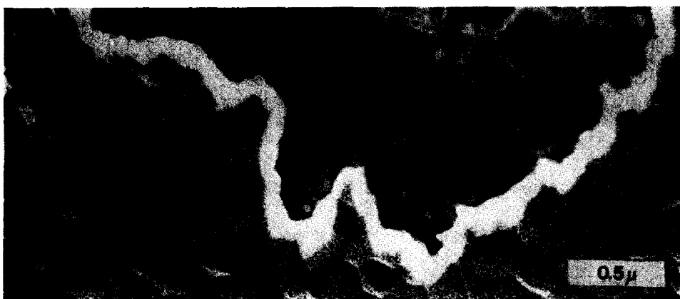
FIG. 3. Electron micrograph of a thin-film specimen reduced for 67 hr at 100^\circ\text{C} and 1 atm \text{H}_2 . Note the excellent parallelism of the \text{Ag}_2\text{S} and Pt phase boundaries. Magnification, 36,000\times .
