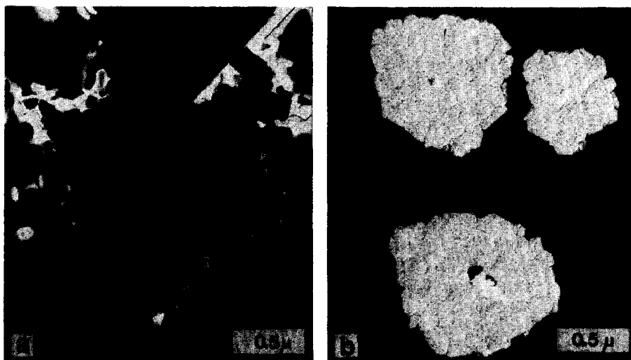
FIG. 4. Electron micrographs of a specimen (a) after a 15-min reduction at 100°C (note that the reduction started at the Pt shadow edge.); (b) after a 2-hr reduction at 100°C. Magnification, 27,000 \times .
